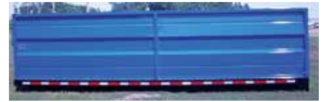
New Grainmaster Body 20' x 102" x 60" Hydraulic Silage Gate, Ladder, 8" Channel Long Sill
