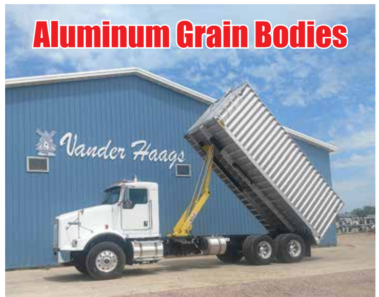
New Grainmaster Body 20' x 102" x 60" Hydraulic Silage Gate, Ladder, 8" Channel Long Sill
